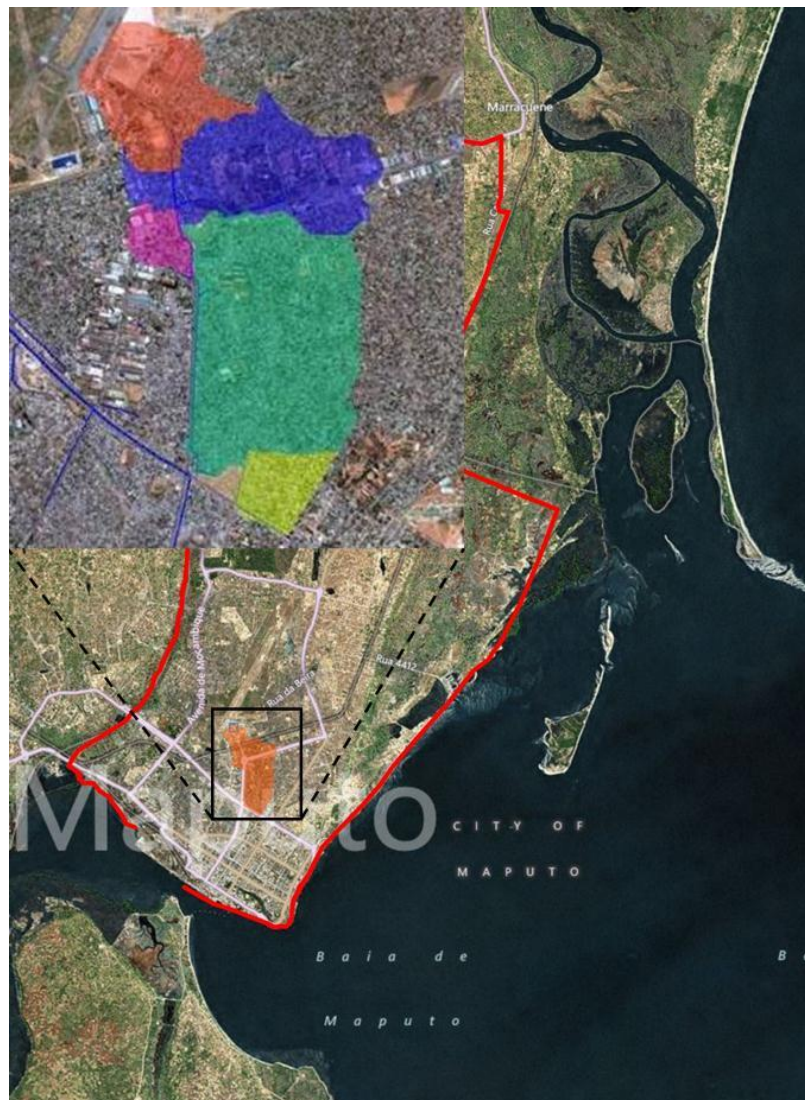
Figure 3-14: Delineation of case study catchment. The “subcatchments” as defined in the SWMM model are shown in different colours.
