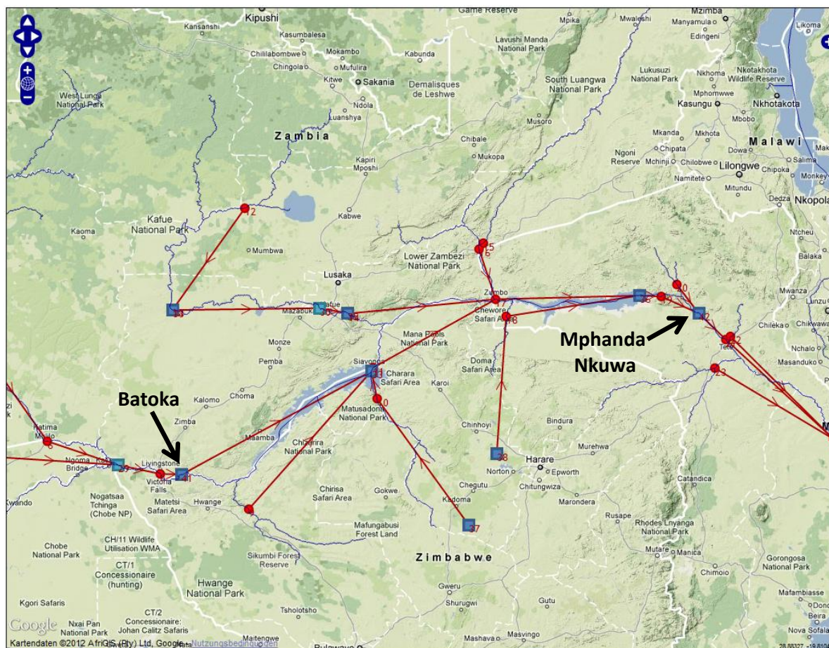
Figure 1-92: Computation point network including the planned reservoirs Batoka Gorge and Mphanda Nkuwa.
