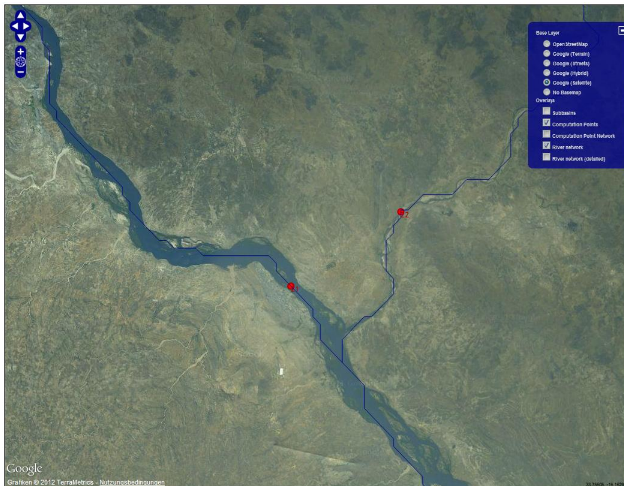
Figure 1-63: Example of Google (Satellite) displayed as base layer in the DSS. Zambezi River and confluence of Revubue River near Tete, Mozambique. Red: computation points. Blue: river network.
