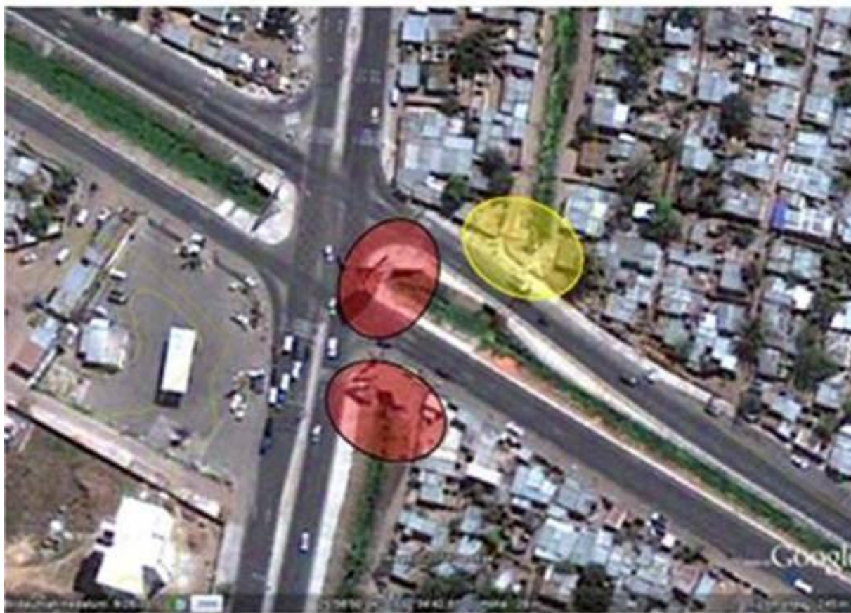
Figure 3-3: Junction of 3 main open channels at the street crossing of Av. Joaquim Chissano / Av. Acordos de Lusaka (yellow circle: outlet of modelled subcatchment; red circles: adjacent culverts with influence on modelled outlet)
